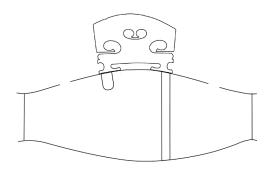
Soundpost placement side to side Equally spaced with the bass bar, inside the bridge foot ~1mm (for violin)
